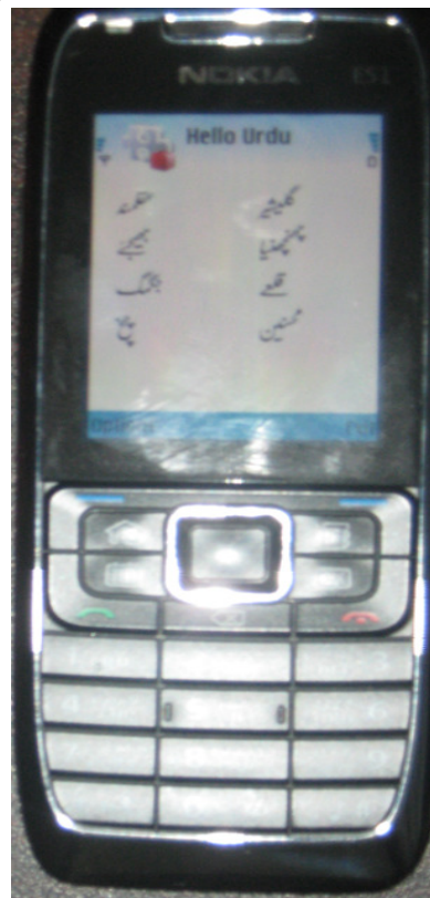
Figure 4: Pango Urdu (Open Type Font Nafees Nastalique) text rendering on a Nokia E51
