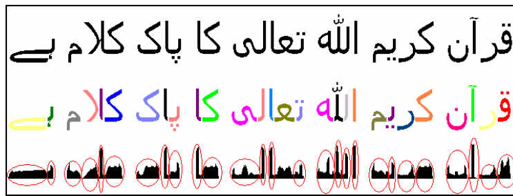
Figure 10 : Histogram and Connection Point Method
